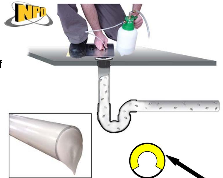
Foam can reach the organic matter that collects in areas like the top and sides of pipes and in the hollow legs of prep tables
